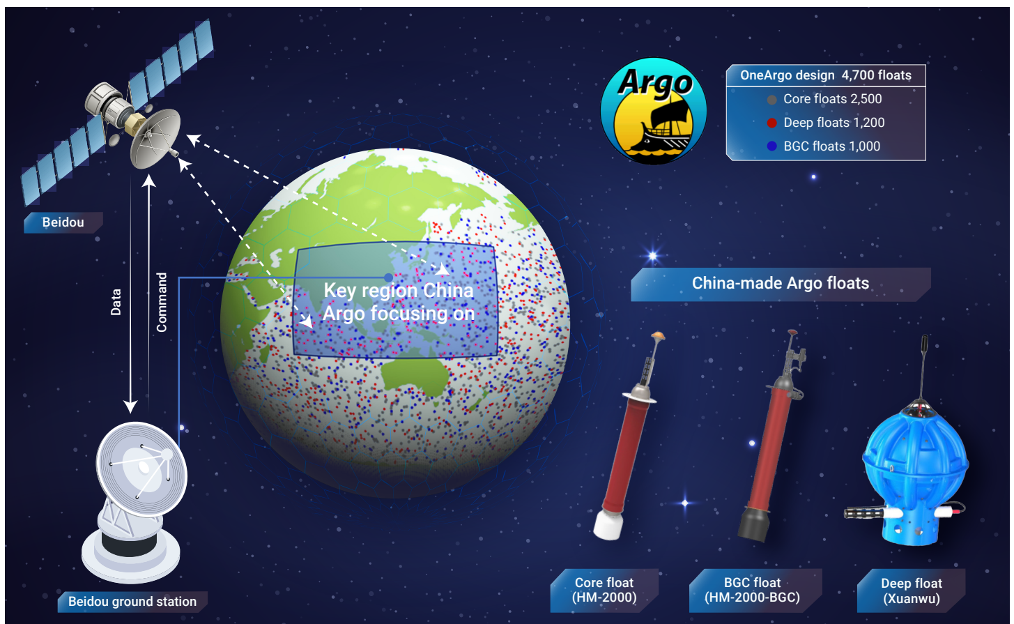
Figure 1. Design for the "OneArgo" array (2,500 core floats, 1,200 deep floats, and 1,000 BGC floats). Shading indicates the key region for future China Argo deployment where a fleet comprising 400 active floats is expected. Prototypes of China's HM-2000, HM-2000 BGC, and Xuanwu floats are superimposed.
