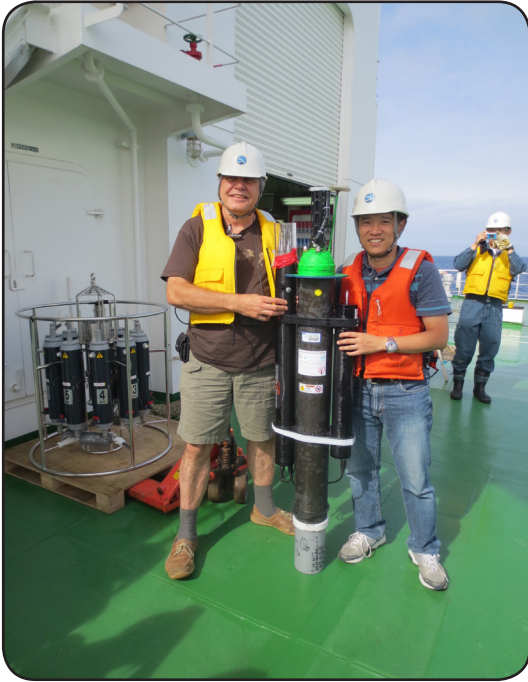
Figure 1: The microstructure float. A MicroRider (RSI Victoria Canada) is mounted on a Navis-Float (SBE).
